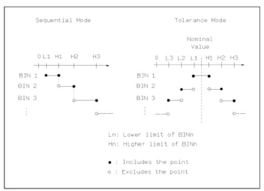
Figure 3-3 Tolerance mode and Sequential mode
