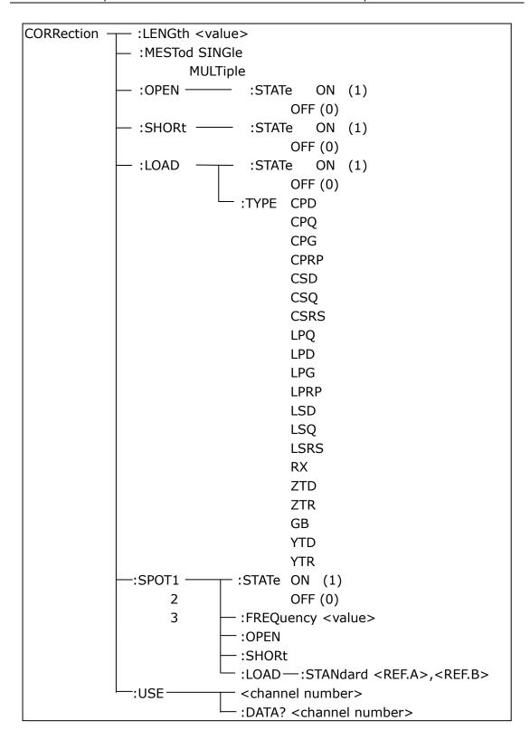
The CORRection:LENGth command is used to set the correction cable length. The CORRection:LENGth? query returns the current set cable length.
