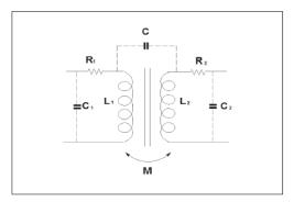
Figure 5-15 Schematic diagram for transformer and its parameter
