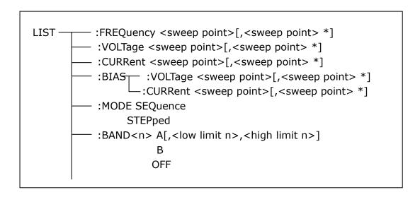
The LIST:FREQuency command is used to clear the original sweep points and set the frequencies of the sweep points. The LIST:FREQuency? query returns the current frequency of each sweep point.
