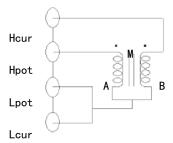
Figure 5-19 Direct measurement method of mutual inductance
