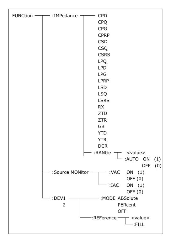
The FUNCtion:IMPedance command is used to set instrument functions. The FUNCtion:IMPedance? query returns the current function parameters.
