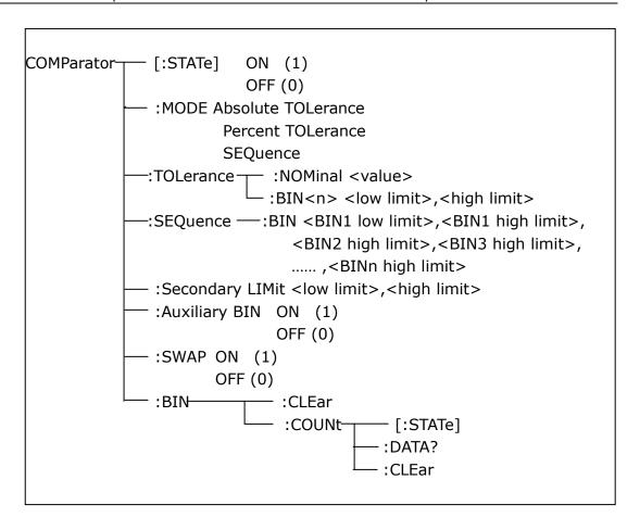
The COMParator[STATe] command is used to set the comparator function as ON or OFF. The COMParator[STATe]? query returns the current comparator state. Command syntax:
