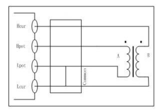
Figure 5-17 Schematic diagram for transformer test connection
