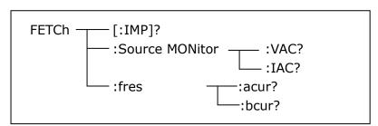
The FETCh[:IMP]? query directs ST2827 to input the last measurement result to the output buffer zone.
