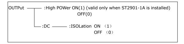
The :HPOWer command is used to set the 1A DC bias source as ON or OFF. The :HPOWer? query returns the current status of the 1A DC bias source. Before using this command, please ensure the option component 1A DC bias source has been installed.
