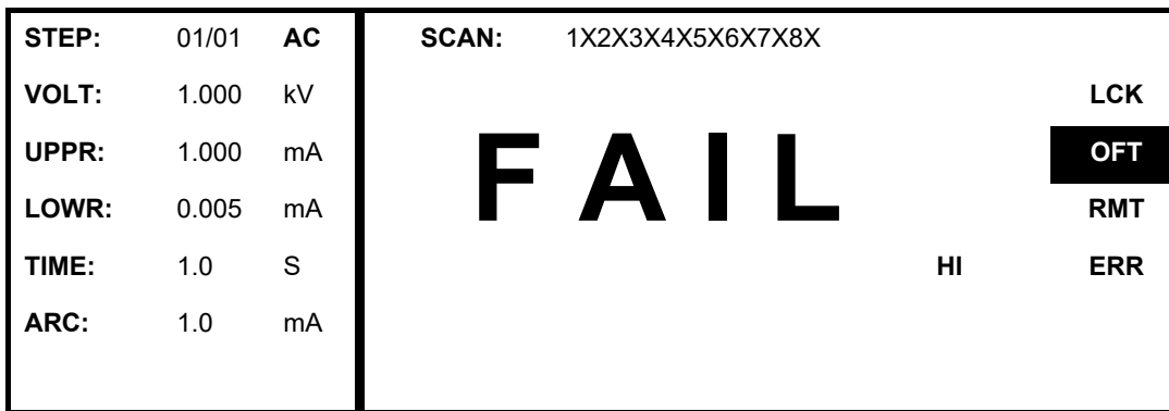
Figure 4-24 Test FAIL Judgement Schematic
