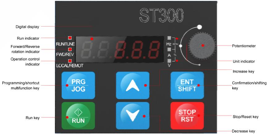
Figure 5-1 Standard LCD keypad
