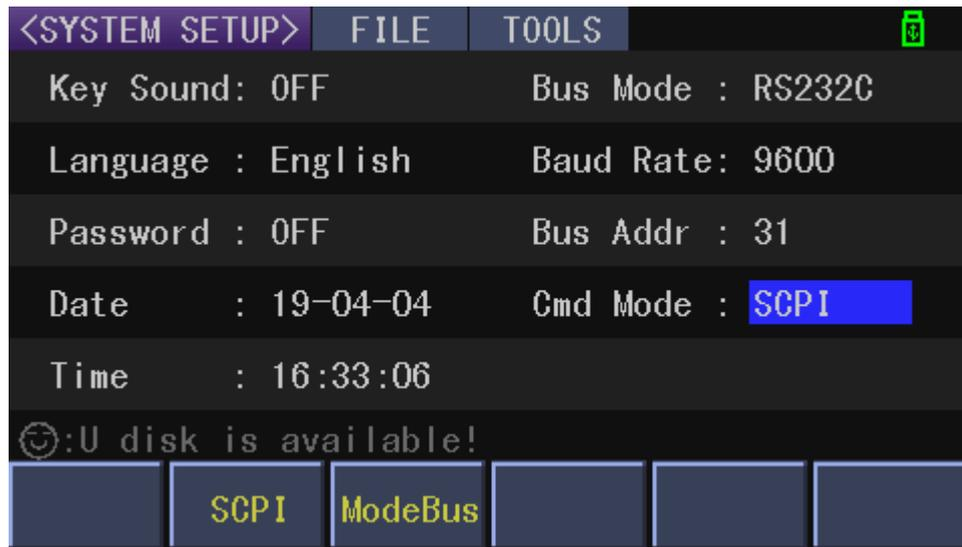
Figure 5-1 System Setup
