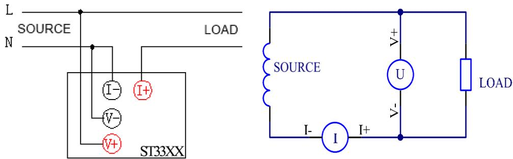
Figure 6-2 External connecting method ----- suitable for large current
