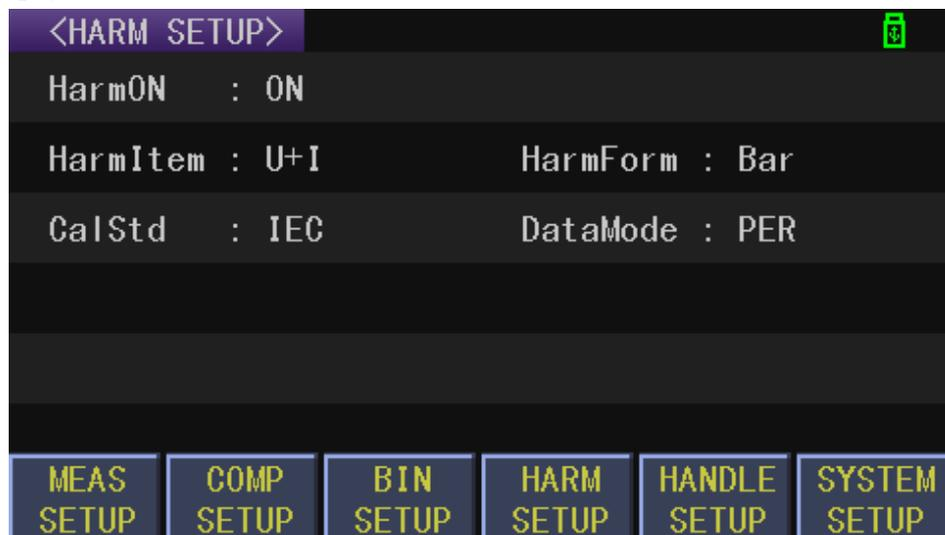
Figure 4-17 Harmonic setup interface
