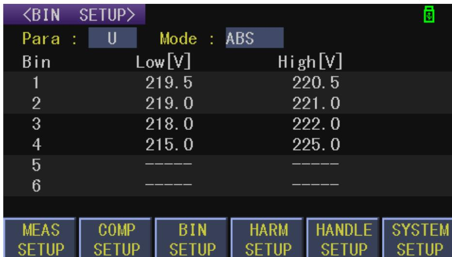
Figure 4-15 BIN setup interface - absolute value mode
