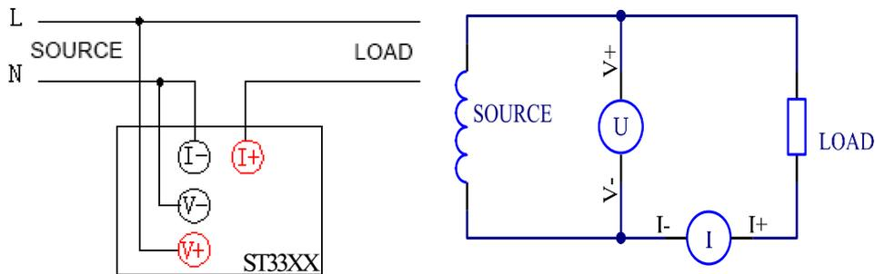
Figure 6-1 Internal connecting method ----- suitable for small current
