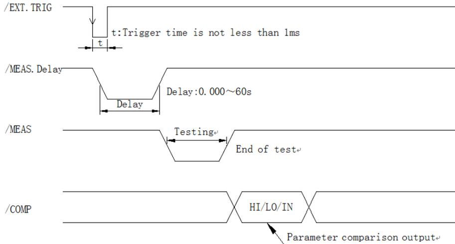
Figure 10-1 Handle timing diagram
