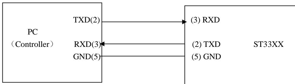
Figure 8-1 Connection of the instrument with PC
