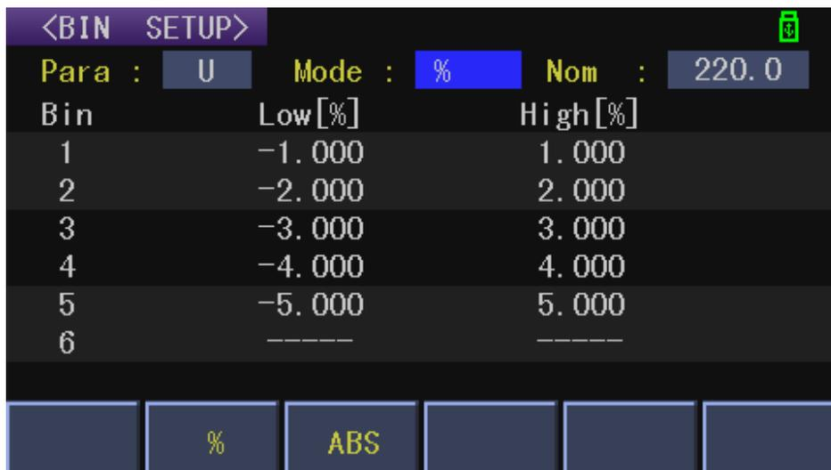
Figure 4-16 BIN setup interface - percentage mode
