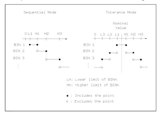
Figure 3-3 Tolerance mode and Sequential mode
