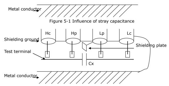
Figure 5-2 Eliminate the influence of stray capacitance
