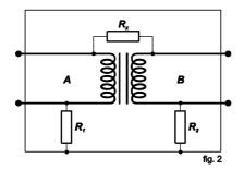
Rx: Insulation resistance between primary and secondary winding.
