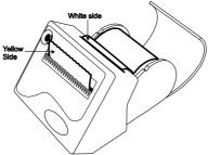
**ATTENTION:** Don't pull the paper, always use the Paper feed key. Never try to put the paper back into the printer. In any of these cases, the printer can be easily damaged.
