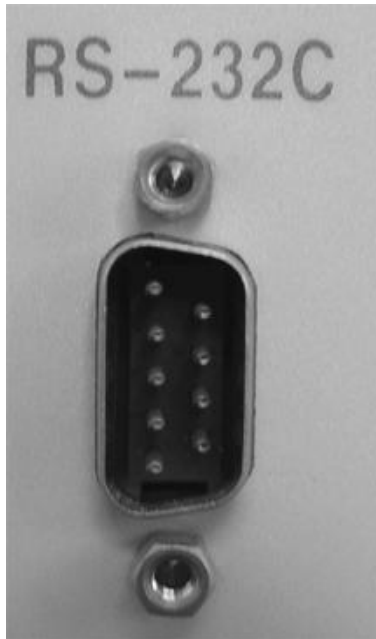
Figure 6-1 Rear Panel RS232 Interface
